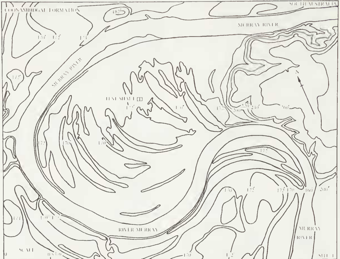
Fig. 39—Map of proposed Chowilla Dam area to show the extreme flatness of the present flood-plain, and the origin of the fossil finds (Fig. 40). Based on S.A. Engineering and Water Supply Chowilla Dam map, whose datum is 106.88 ft. below mean sealevel, Adelaide. The contours are in feet. Thus although the Murray River at the downstream end of this map is c. 390 miles (628 km) from the sea, it is only of the order of 53 ft. (16 m) above sealevel. Site 1.
